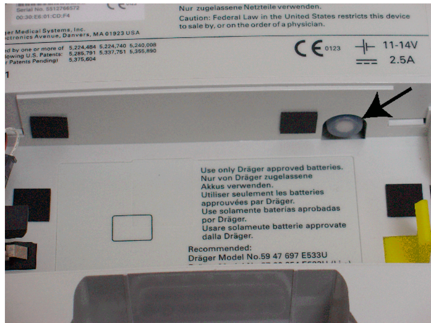
Figure 1 Location of NBP Air Intake Filter in Battery Compartment
